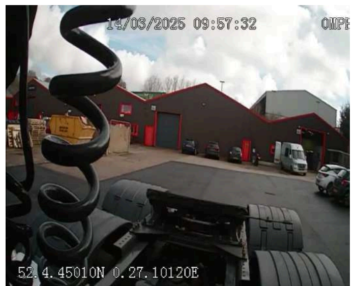
5th Wheel Camera View to assist with height of kingpin
