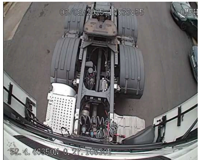
5th Wheel Camera View to assist with height of kingpin
